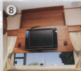
8 TV CABINET The flatscreen TV can be concealed neatly in its hinged locker when not in use. It's a simple alternative to sliding mechanisms or brackets
